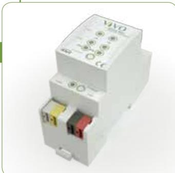
The KNX/IP SPICA KNX interface is a Tunneling device that allows to couple an Ethernet line with a bus KNX line. Thanks to its flexibility, the device can be used as programming interface through the IP Network (even remotely\*) and it can manage up to four parallel connections which makes it suitable for use also as gateway for the supervision systems.
