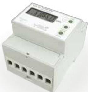
Nunki KNX is an active energy meter for three phase alternating current, with direct connection up to 63 A. The device features 2 impulse outputs for active and reactive energy, measured according to two different tariffs. Nunki KNX has a 9-digit LCD.
